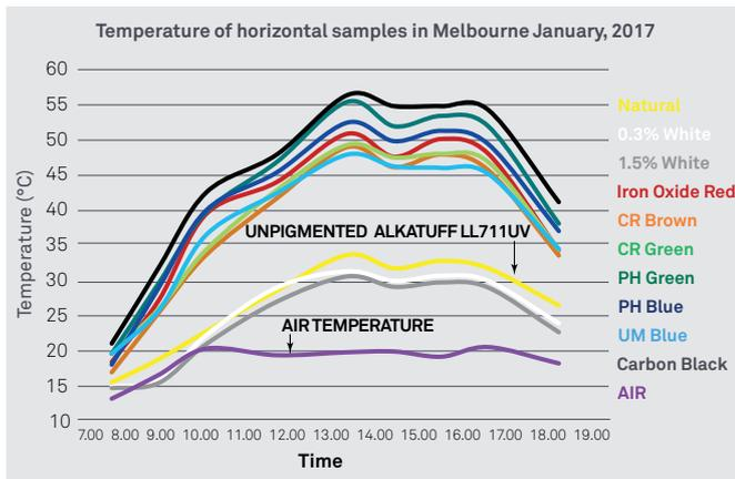
**Figure 8.** The different pigments generate different amounts of heat
