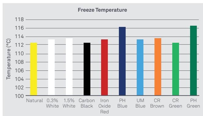
Figure 4. Freeze temperature test results
