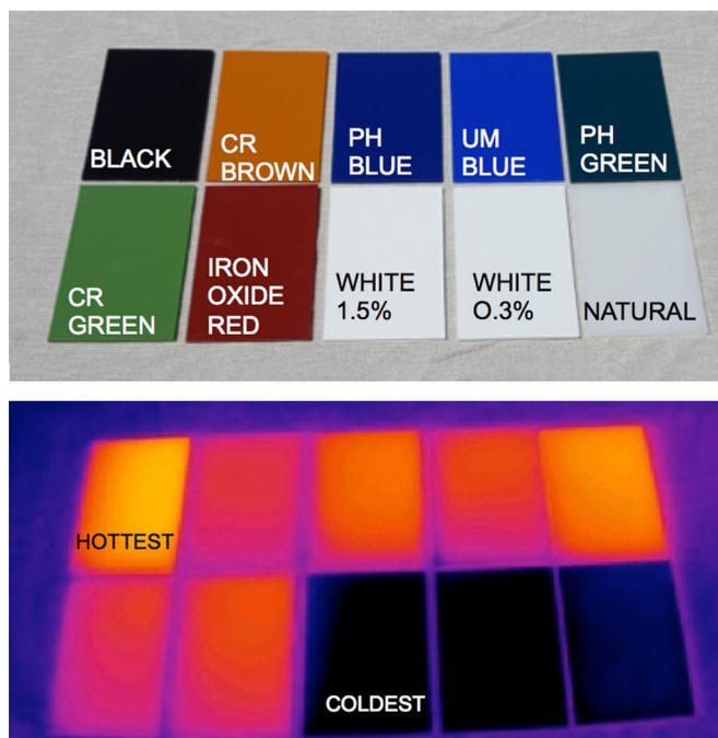
Figure 7. Thermal imaging of different pigments
