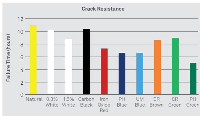
**Figure 2. Crack resistance test results**
