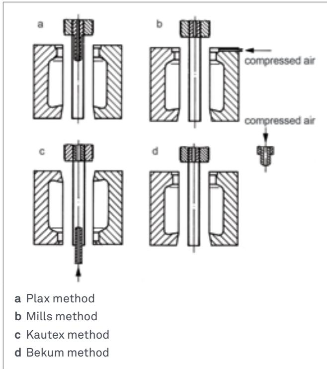
**Figure 38: Blowing Methods Named After the Inventor or Machine Manufacturer**
