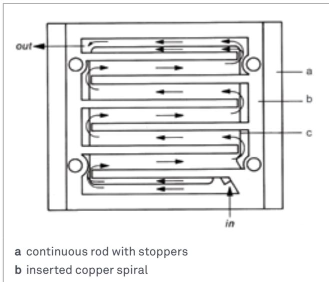
**Figure 25:** Cooling Channels with Labyrinth-type Water Flow
