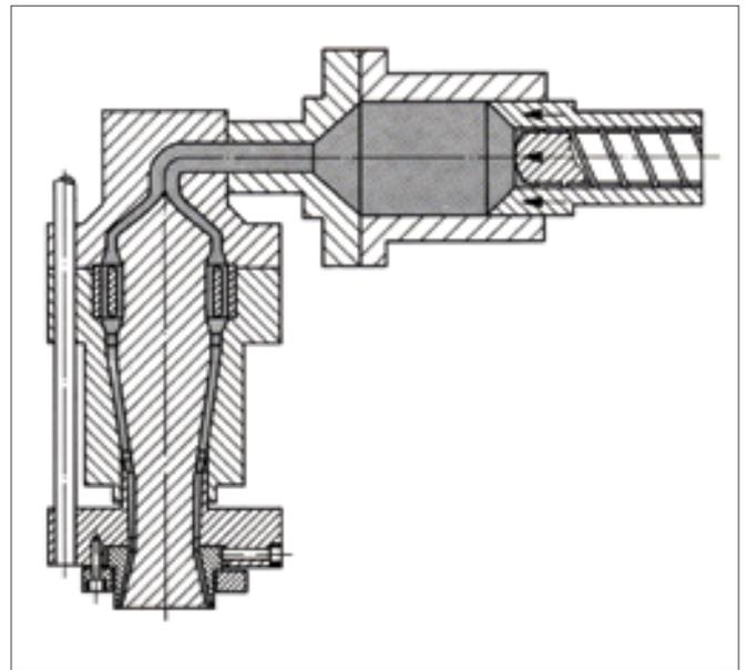
Figure 14: Reciprocating Barrel Accumulator (design: J. Fischer, Lohmar)
