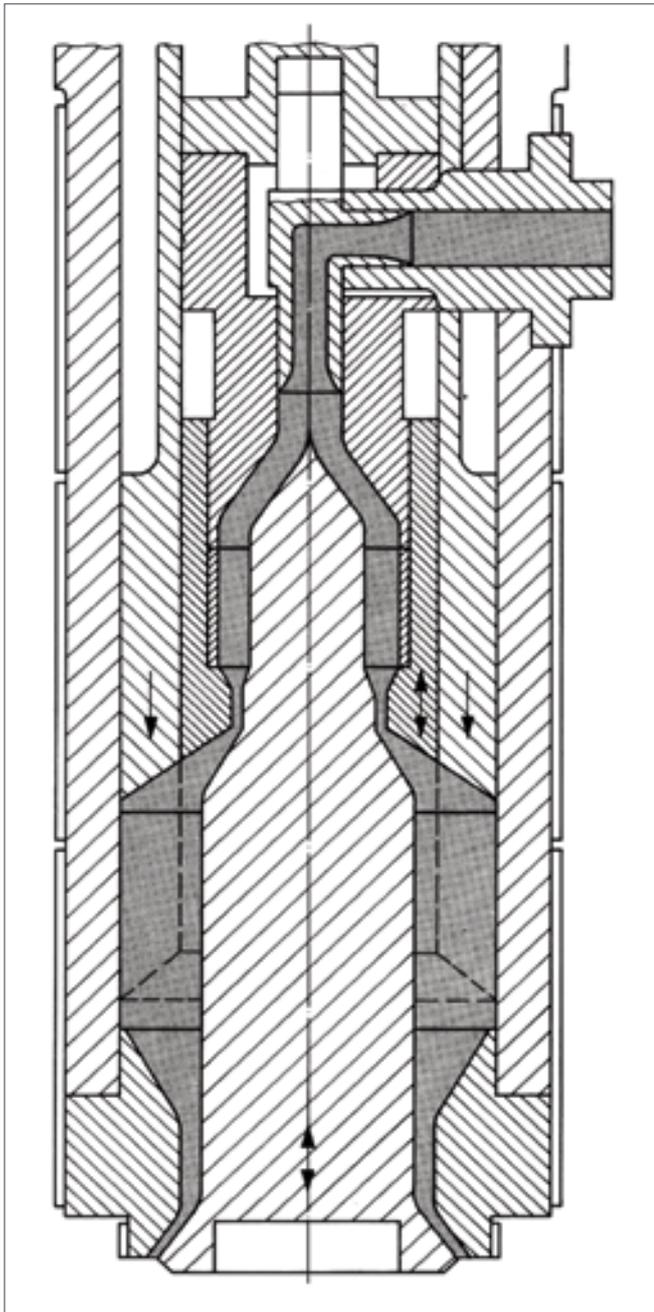
**Figure 21: Tubular Plunger Accumulator**
