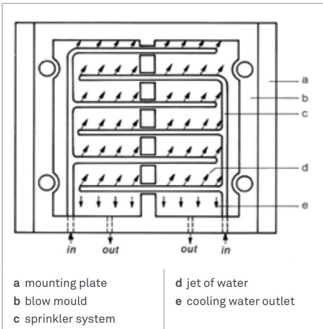
**Figure 28: Sprinkler (boundary layer) Cooling**
