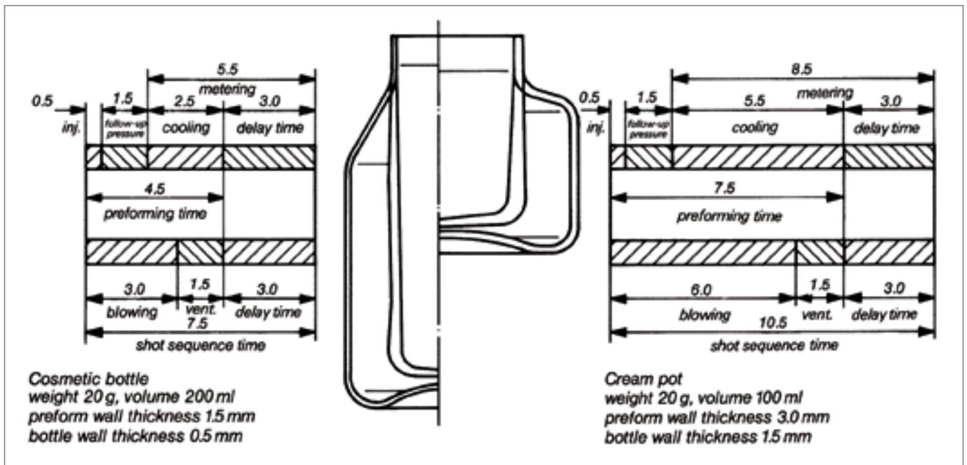
Figure 60: Shot Sequence Time as a Function of Pre-form Wall Thickness at Constant Article Weight
