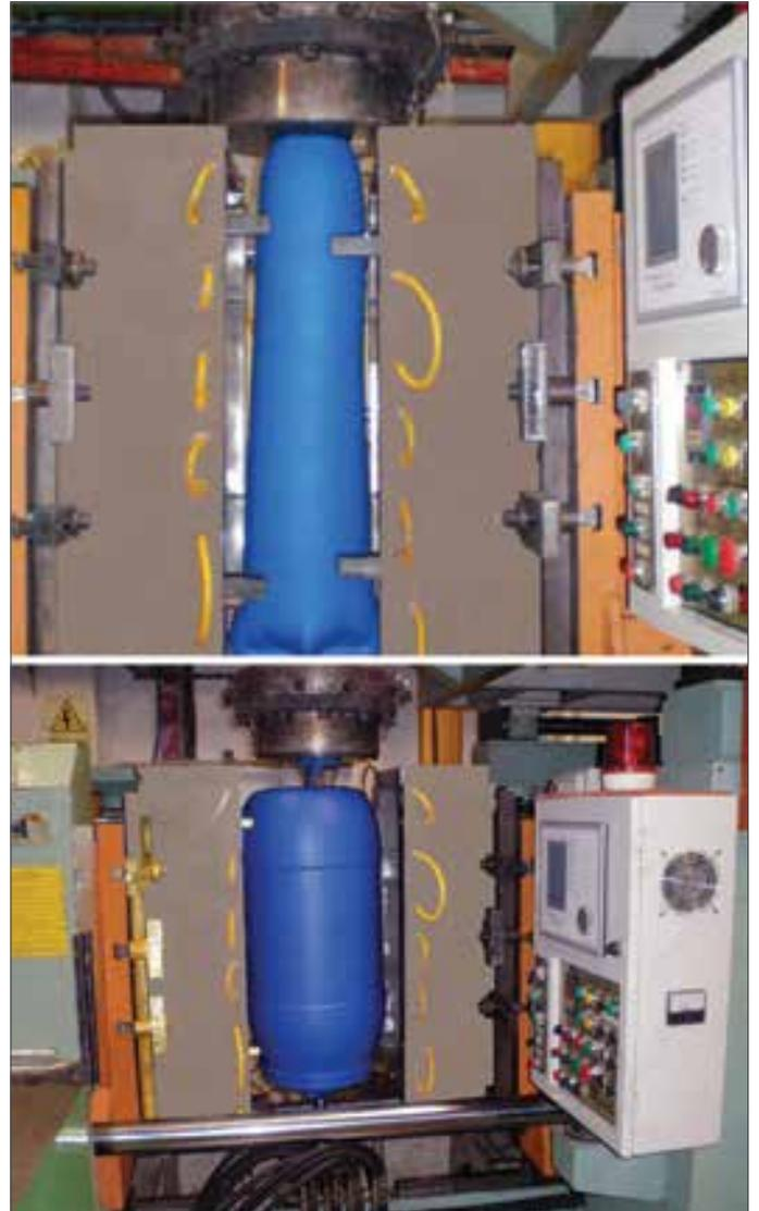
Figure 15b: Ram Accumulator used to Blow Mould Large Volume Drum
