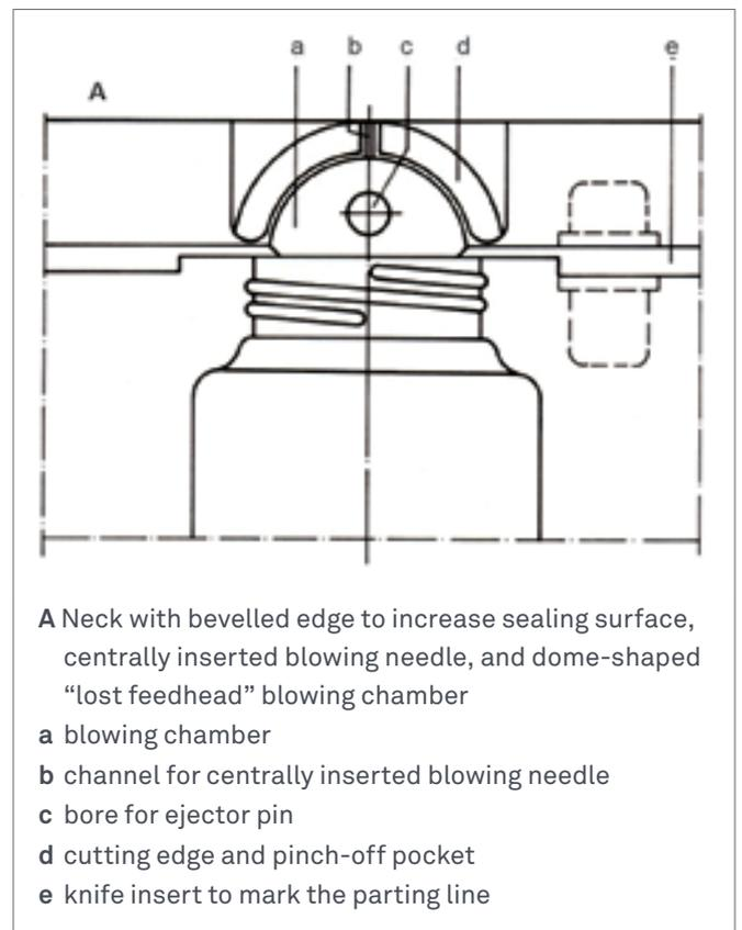
**A** Neck with bevelled edge to increase sealing surface, centrally inserted blowing needle, and dome-shaped “lost feedhead” blowing chamber
