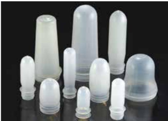
**Figure 49b:** Collection of Injection Moulded "Pre-forms" Awaiting Blow Moulding into Containers
