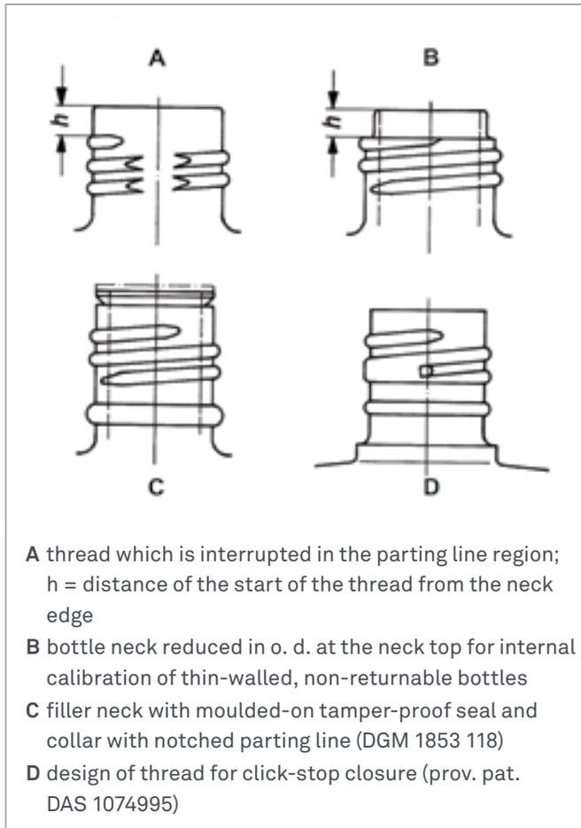
**Figure 42: Design of Thread and Neck for Bottles**
