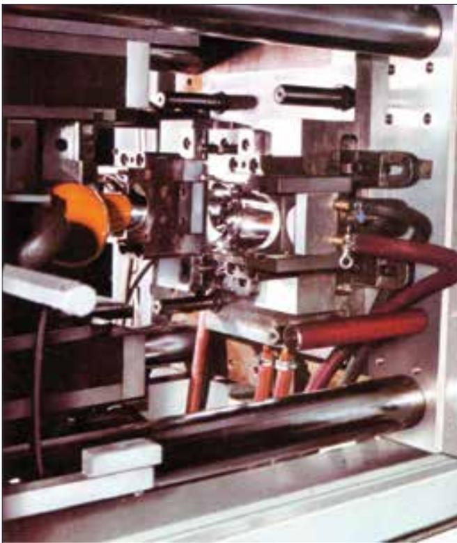
**Figure 51:** Injection Blow Mould Machine
