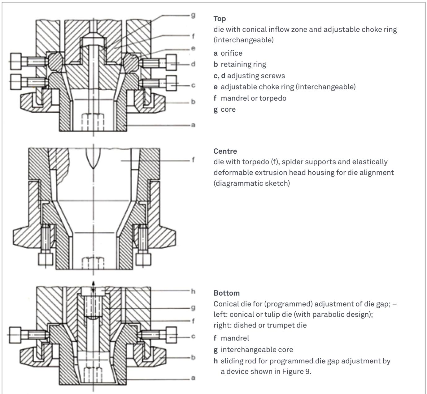
Figure 11: Conical Dies
