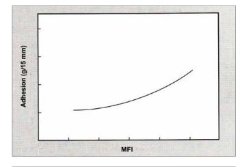
**Figure 10:** Effect of MFI on Adhesion of Extrusion-Coated LDPE to Porous Substrates
