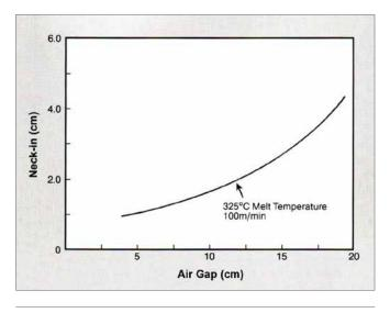
Figure 8: Typical Effect of Air Gap Distance on Neck-in
