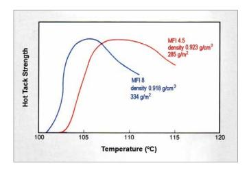
**Figure 17:** Typical Hot Tack Strength Characteristics of *Alkathene* LDPE Extrusion Coating Polymers.
