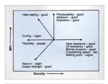
**Figure 1:** Influence of MFI and Density of Low Density Polyethylene on Processability and Laminate Properties
