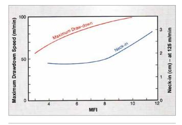
Figure 5: Variation of Drawdown and Neck-in Performance for *Alkathene* LDPE Resins of Different MFI
